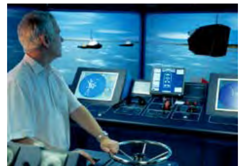
Bridge simulator cubicle equipped with hands-on control for a Voith Schneider tug model.
